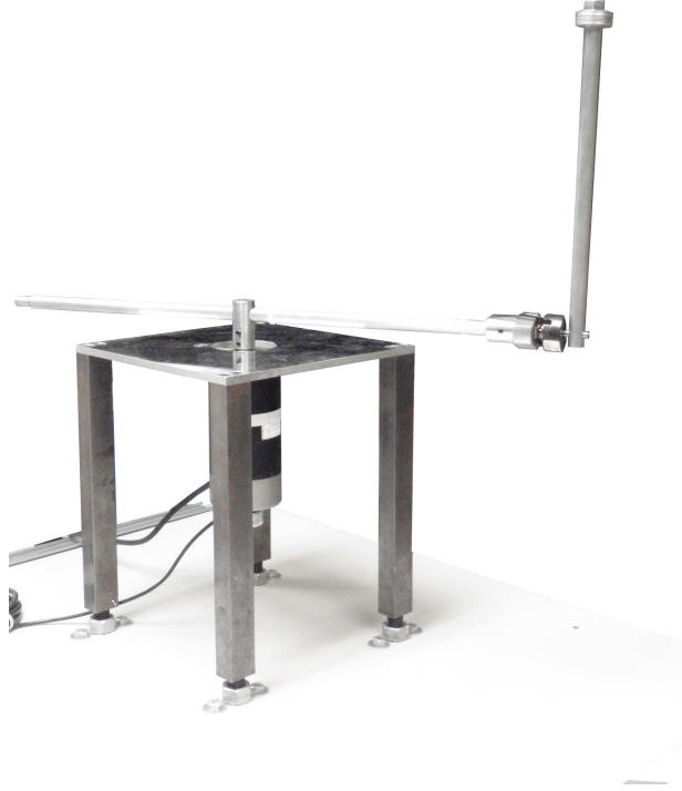
Fig. 2. Furuta pendulum prototype built at Instituto Politécnico Nacional–CITEDI Research Center.
